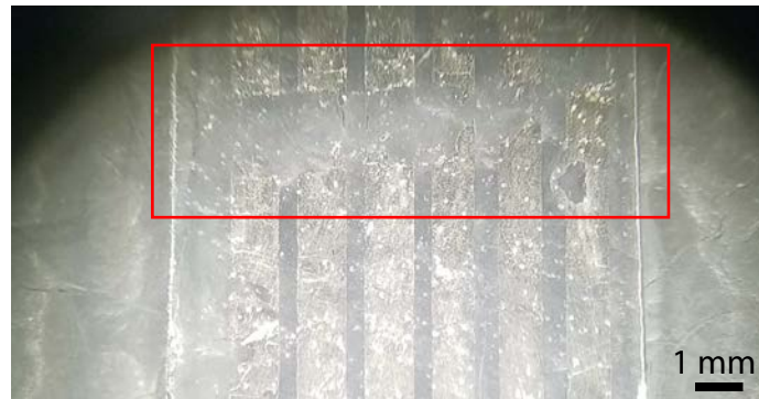
Figure 2.12: Sample microscope image of inkjet printed electrode traces. Close visual inspection can illuminate fabrication errors such as the open circuits in the outlined region. Image taken with 10x magnification.
