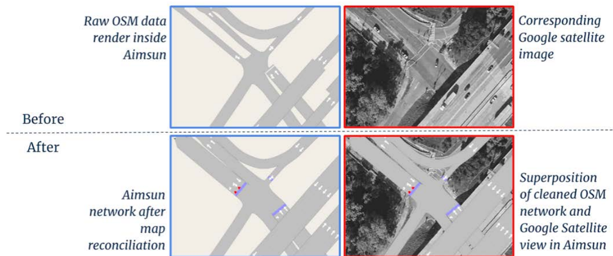
Figure 5.2: Before and after manual editing of the OSM network in Aimsun with comparison to the Google Satellite image.
