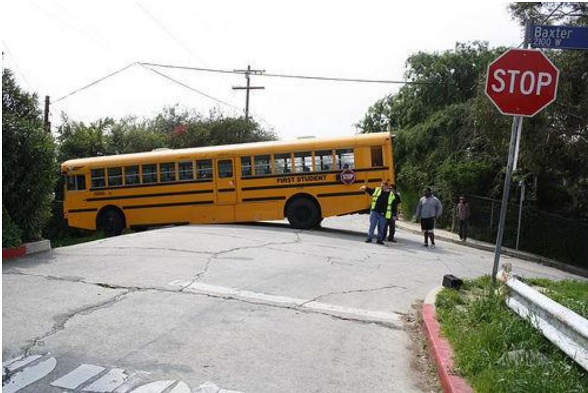
Figure 4.9: Image of a bus crash because it was routed on a too steep road. Photos by Ingrid Peterson via Flickr.
