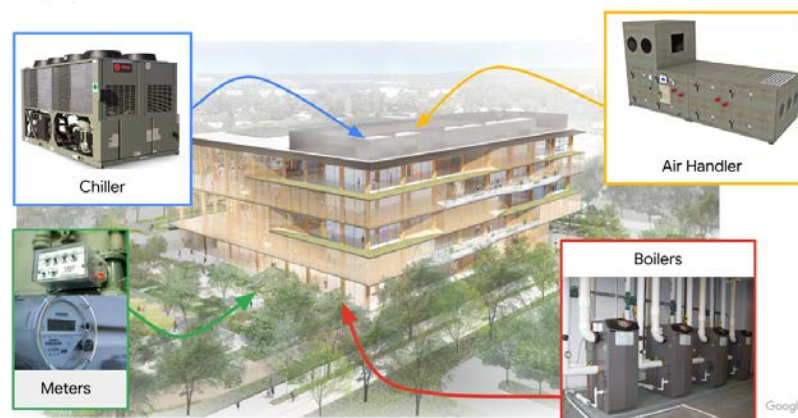
(a) Depiction of AHU, Boiler, Meters, and Chillers.
