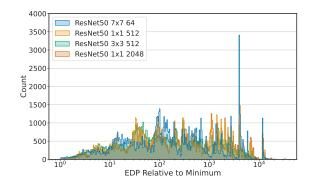
Figure 2.2.1: A histogram of energy-delay product (EDP - left is better) values for 100K randomly sampled valid mappings for BERT (matmul-dominated kernel, left) and Resnet50 (convolution, right), simulated on Timeloop [71]. Note that the x-axis is log-scale. Only a minuscule fraction of mappings, on the far left of each graph, provide acceptable performance for each processor.
