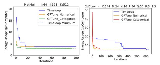
Figure 6.2.1: Energy (lower is better) attained by Timeloop's brute-force mapper and GP-Tune for matrix multiplication (left) and 2D convolution (right). GPTune was run for 100 iterations; the best value found is indicated with dotted line extending to the right.
