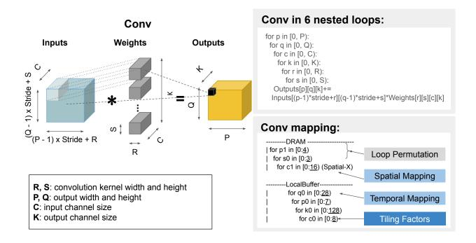
Figure 2.2.2: Mapping representations for matrix multiplication and convolutions. Originally published in [50]
