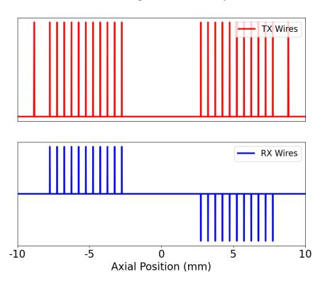
Figure 6.5: TX/RX Wiring Solution given by the Linear Program. The LP provided a solution that adds a few extra winding towards the edges of the coil. Not seen are the partial windings also offered by the solution.
