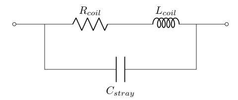
Figure 3.1: Circuit model of receive coil includes the inductance  $L_{coil}$ , equivalent series resistance  $R_{coil}$ , and stray capacitance  $C_{stray}$ . For the purposes of noise integration and analysis, we only consider the inductance and resistance.
