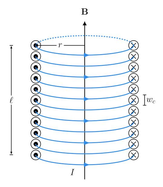
Figure 2.2: Cross section of typical solenoid receiver coil used in MPI where  $\ell$  is the length of the coil, r is the radius of the coil,  $w_c$  is the coil gauge, I is the current, and  $\mathbf{B}$  is the magnetic field generated by the current-carrying wire.
