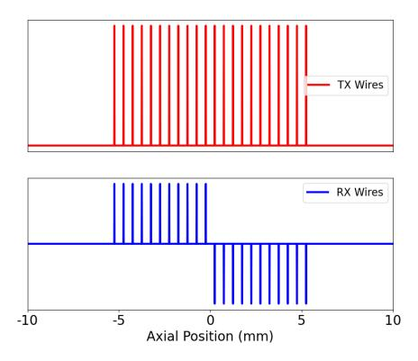
Figure 6.3: TX/RX Wiring of Intial Gradiometer Coil Pair with no gap between the pair.
