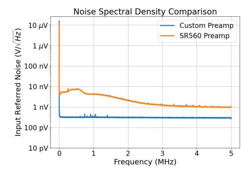
Figure 3.9: Custom optimized preamplifier achieves  $e_n = 300 \,\mathrm{pV/\sqrt{Hz}}$ , more than a 10-fold improvement over the SR560's  $e_n = 3.4 \,\mathrm{nV/\sqrt{Hz}}$  over a wider bandwidth. Data was collected with a spectrum analyzer and the inputs to the amplifier shorted.
