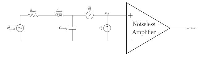
Figure 2.4: The Two-Port Noise Model now includes the coil inductance and stray capacitance. This presents a challenge when noise matching because the current noise contribution increases with frequency due to the frequency dependent impedance of the coil.
