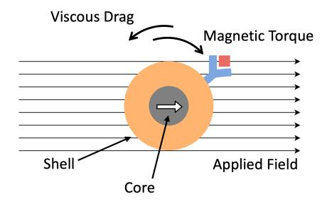
Figure 1.9: Brownian relaxation can be used to sense changes in viscosity, temperature, or binding effects for contrast.
