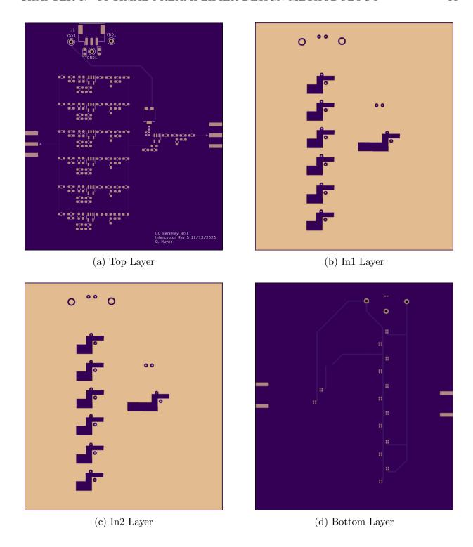
Figure 3.6: Layout of Preamplifier PCB. In Figs. 3.6b and 3.6b, the ground planes were removed from the inverting input nodes of the amplifiers to reduce parasitic capacitance and prevent instability. In Figure 3.6d,  $0.1\,\mu\text{F}$  and  $0.01\,\mu\text{F}$  decoupling capacitors were placed close to the supply pins of the amplifiers.  $10\,\mu\text{F}$  tantalum capacitors were placed closer to the power inputs of the board.
