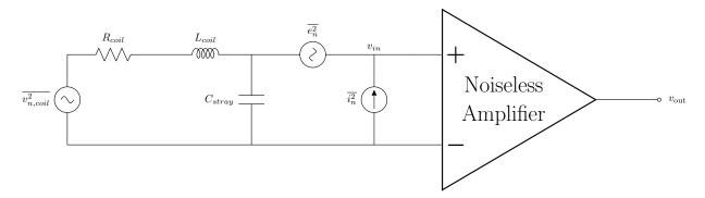
Figure 3.2: Noise model of receive coil and preamplifier includes the inductance  $L_{coil}$ , equivalent series resistance  $R_{coil}$ , and stray capacitance  $C_{stray}$ . For the purposes of noise integration and analysis, we only consider the inductance and resistance. It now also includes the preamplifier's input referred voltage  $e_n$  and current noise  $i_n$ .
