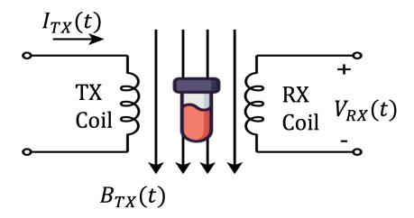
Figure 5.1: Excitation of particles requires simultaneous TX/RX
