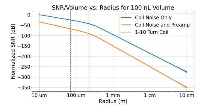
Figure 4.5: For  $100\,\mathrm{nL}$  volume the SNR/volume shows a  $40\,\mathrm{dB/dec}$  slope for  $r < 300\,\mathrm{\mu m}$  for the coil and preamp model versus  $30\,\mathrm{dB/dec}$  for the coil only model. This shows that the preamplifier noise is dominant in this model.
