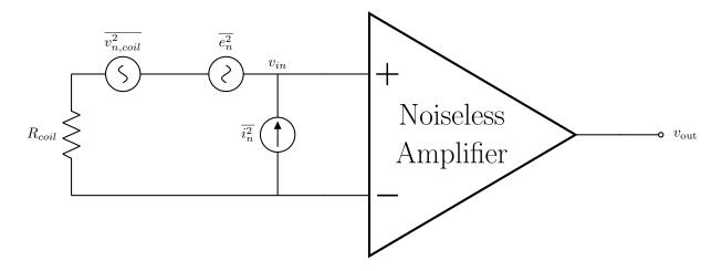
Figure 2.3: The Two Port Noise Model for a Resistive Sensor includes input referred voltage noise  $e_n$  and input referred current noise  $i_n$  modelled outside the amplifier, which is now considered "noiseless." This model simplified noise factor calculations for analysis and optimal noise matching.
