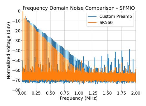
Figure 3.11: Improved bandwidth of the custom optimized preamplifier exposes more of the harmonics in SFMIO signal acquisition. The scan parameters were  $f_0 = 20 \,\mathrm{kHz}$ , 20 mT sinusoidal excitation for 0.25 seconds. Even with shielding, the AWR's receiver unfortunately still acts as a great pickup coil for other EMI sources such as local AM radio stations. Further shielding can be done by placing the receive frontend in a Faraday cage.
