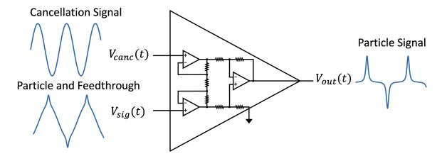
Figure 7.2: The instrumentation amplifier can cancel signals common to both inputs. If the direct feedthrough can be captured, generated as a cancellation signal, and fed into the other input, then the difference amplifier can output the difference  $V_{out}(t) = V_{sig}(t) - V_{canc}(t) = V_{spio}(t) + V_{ft}(t) - V_{ft}(t) = V_{spio}(t)$  allowing us to capture just the particle signal.
