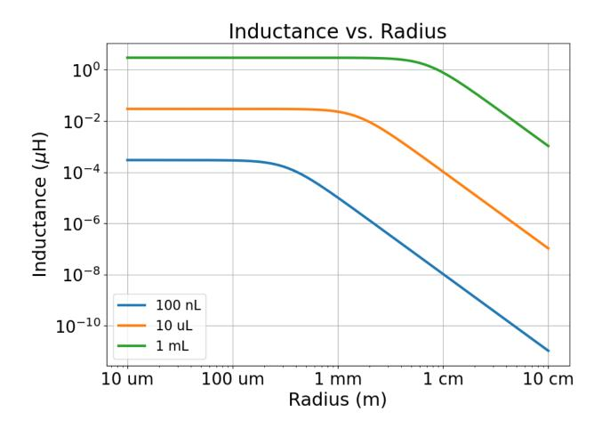
Figure 4.3: Decreasing radius shows an increase in coil inductance up until a certain point when the inductance is constant. This regime is when  $r \ll \sqrt[3]{\frac{10V}{9\pi}}$ . This is due to the long solenoid approximation where  $r \ll \ell$  and the coil inductance no longer is strongly dependent on radius
