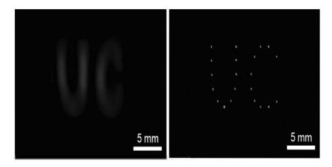
Figure 1.5: (Right) SFMIO particle tracers in an *in vitro* 2D scan taken with our group's 7 T/m Field Free Line projection scanner experimentally show higher resolution and sensitivity compared to (Left) conventional SPIOs.
