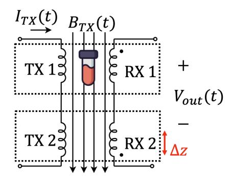
Figure 5.3: A gradiometer can be constructed by winding two coils in anti-series, where one coil is wound in the opposite direction of the other.
