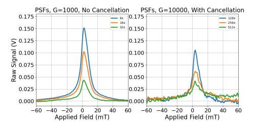
Figure 7.11: Point spread functions (PSFs) of diluted samples of Vivotrax ( $40\,\mu\text{L}$  of  $5.5\,\text{mg/mL}$  stock concentration). With active cancellation, we are able to detect 10-fold smaller masses of iron at the same signal level, showcasing an improved dynamic range. At lower amounts of iron, we start to see the thermal noise of the system, achieving thermal noise dominant LOD.
