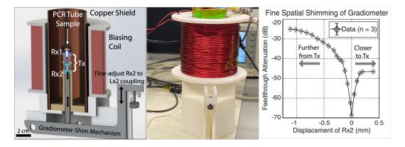
Figure 5.4: (Left) CAD model of the gradiometric cancellation coil shows the cantilever mechanism used to shim the relative distance between the receive coils. (Middle) Constructed gradiometric coil system as part of building the next generation Arbitrary Waveform Relaxometer. (Right) Coils are sensitive in mechanical placement, with nearly 10 dB feedthrough attenuation per 50 µm near the ideal placement point.
