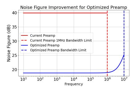
Figure 3.4: Simulations show that the optimized custom preamplifier with N=5 parallel unit amplifiers achieves more than a ten-fold SNR boost (20 dB noise figure improvement) across the desired receive bandwidth.
