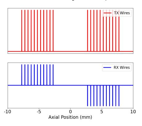
Figure 6.4: TX/RX Wiring of Intial Gradiometer Coil Pair with a gap equal to the radius of the coils between the pair.
