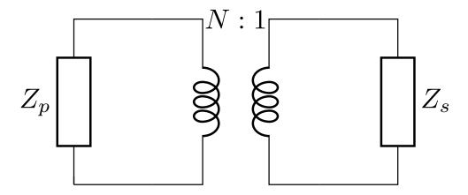
Figure 2.5: Transformers transform the impedance of the primary to the secondary and is one method in noise matching and impedance matching.
