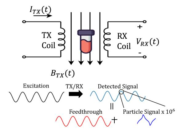
Figure 7.1: Particle Excitation creates direct feedthrough interference. A transmit coil is driven with a current waveform which generates the excitation field. The detected signal is a combination of both the nanoparticle signal and induced voltage from the transmit to receive coil coupling. This feedthrough interference is much larger than the particle signal.
