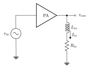
Figure 8.1: Power Amplifier driving transmit coil, which can be modelled as an inductive load with series resistance.
