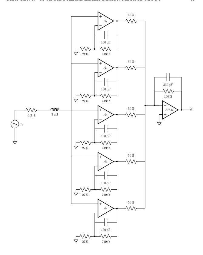
Figure 3.7: The optimal design metholodogy yields a preamplifier circuit that with 5 parallel amplifiers in the first stage. The second stage is an inverting summing amplifier with gain of 10. Capacitors were placed in shunt with the feedback resistors of each stage to set a low-pass filter cut-off frequency at 5 MHz.
