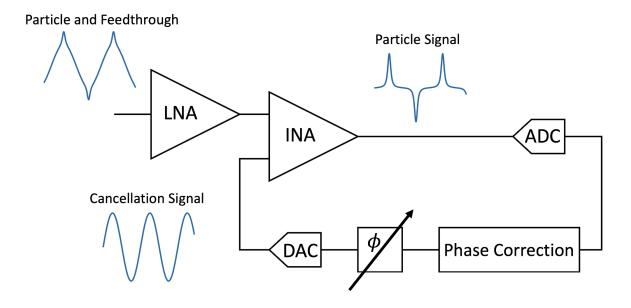
Figure 7.6: The complete receive system architecture is shown as follows. The receive coil picks up the desired particle signal and undesired feedthrough. Both components are amplified by the LNA. The instrumentation amplifier (IA) takes the generated cancellation signal and subtracts it from the LNA's output, resulting in only the desired particle signal going into the ADC.
