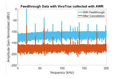
Figure 5.5: Constructed gradiometer for the next generation AWR achieves 71 dB attenuation of direct feedthrough.
