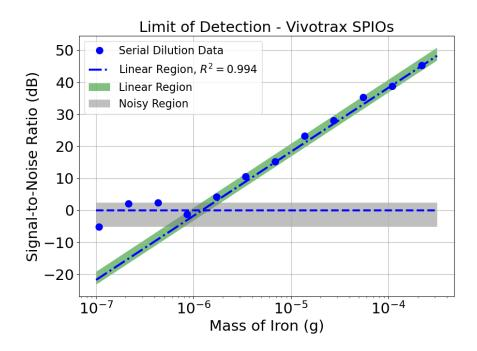
Figure 7.10: Samples of Vivotrax ( $40\,\mu\text{L}$ , 5.5 mg/mL stock concentration) were serially diluted up to 2048x and analyzed with the AWR. The resulting limit of detection curve shows a linear dependence of the signal to mass of iron down to  $1\,\mu\text{g}$  for an acquisition time of 0.3 seconds (no averaging).
