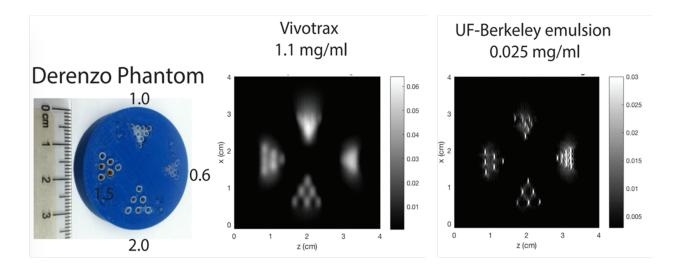
Figure 1.4: (Right) Newer SFMIO particle tracers show higher resolution and sensitivity per mass of iron compared to (Middle) conventional SPIOs.
