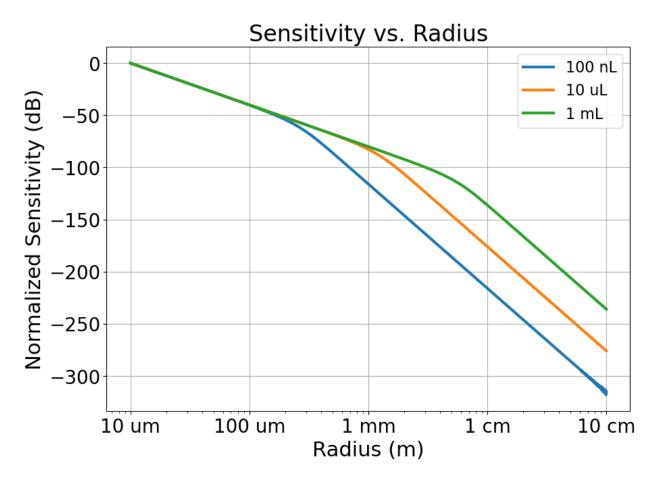
Figure 4.2: Decreasing radius shows a 40 dB/decade increase with sensitivity. Note that this regime is only when  $r \ll \sqrt[3]{\frac{V}{\pi}}$ . Outside this regime, the sensitivity of the coil per volume is weaker.
