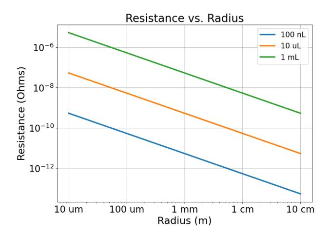
Figure 4.4: Coil resistance increases linearly with decreasing r.
