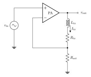
Figure 8.2: Power Amplifier driving transmit coil in feedback sets the current through the coil to be directly proportional to the input voltage,  $I_{tx} = \frac{V_{in}}{R_{set}}$ . Care must be taken in compensating the feedback network to prevent unwanted oscillations.
