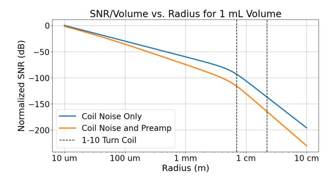
Figure 4.7: For  $100\,\mathrm{nL}$  volume the SNR/volume shows a  $40\,\mathrm{dB/dec}$  slope for  $r<4\,\mathrm{mm}$  but tapers down to  $30\,\mathrm{dB/dec}$  for the coil and preamp model versus  $30\,\mathrm{dB/dec}$  for the coil only model. This shows that the preamplifier noise and coil noise have relatively equal contributions in this model.
