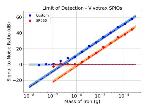
Figure 3.10: 20 mT 20 kHz sinusoidal excitation for 0.25 second acquisitions of serial dilution of VivoTrax<sup>TM</sup>show that the custom preamplifier board achieves roughly 200 ng iron limit of detection whereas the SR560 only achieves 1 µg. This experimentally confirms the 5-fold boost in SNR from optimal noise matching. This experiment also confirms that with just 25 seconds of averaging, our AWR design should detect roughly  $200 \text{ng}/\sqrt{25s/0.25s} = 20 \text{ ng}$  of SPIOs.
