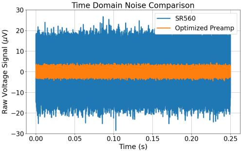
Figure 3.8: Constructed Preamp PCB shows a factor of more than 4 decrease in noise. Input referred integrated noise of the optimized preamplifier was measured to be  $0.9\,\mu\mathrm{V}$  whereas the SR560 preamplifier measured  $5.2\,\mu\mathrm{V}$  noise.
