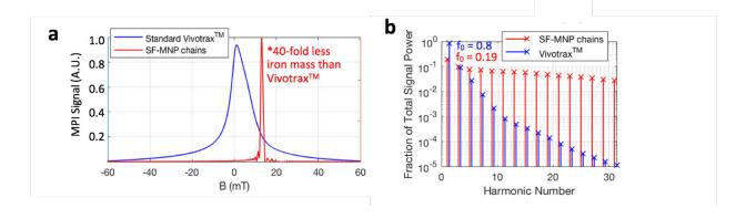
Figure 1.6: (a) Newer SFMIO nanoparticle tracers exhibit sharper magnetic transitions and lend to higher resolutions compared to conventional SPIOs, as shown in the point spread functions. (b) Under sinusoidal excitation, the SFMIO signal spectra is richer in harmonics, requiring a 10-fold wider receive bandwidth. Images were reproduced with permission from [5].
