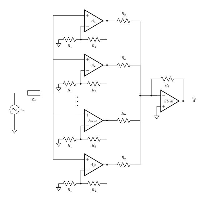
Figure 2.8: Using N parallel amplifiers provide  $\sqrt{N}$  improvement in voltage noise and a concomitant increase in current noise. This means the effective noise power,  $p_n$ , remains constant. A summing amplifier in the second stage sums the N signals. We can use the number of parallel amps, N, as a free design parameter to optimize noise figure.
