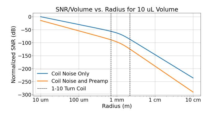
Figure 4.6: For  $100\,\mathrm{nL}$  volume the SNR/volume shows a  $40\,\mathrm{dB/dec}$  slope for  $r < 1.5\,\mathrm{mm}$  for the coil and preamp model versus  $30\,\mathrm{dB/dec}$  for the coil only model. This shows that the preamplifier noise is still dominant in this model.
