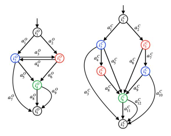
Figure 6.1: Example of a single-origin single-destination original network  $G_O$  (top left, with superscript O), and its corresponding condensed DAG, or CoDAG, representation G (top right, with superscript C). Arc correspondences between the two networks are given by Table 6.1, while node correspondences are indicated by color.
