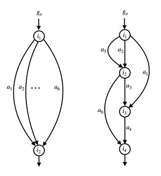
Figure 7.1: (Left) A parallel arc-network with 6 arcs; here,  $i^* = i_1$ . (Right) A more general network with 6 arcs; here,  $i^* = i_2$  since there exists two routes from  $i_2$  to the destination  $i_4$  which do not share an arc.
