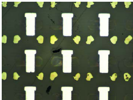
Figure 2.4: (a) Optical microscopy of OTFTs with evaporated aluminum gates.
