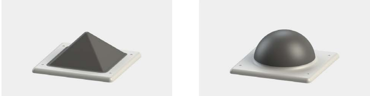
Figure 5.9: Pyramid and hemisphere molds used for software calibration. Two test structures were developed and used to calibrate the software toolkit.
