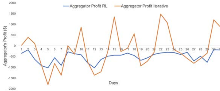
Figure 7.4: Comparing aggregator profit for market solving prices with iterative pricing and RL controller
