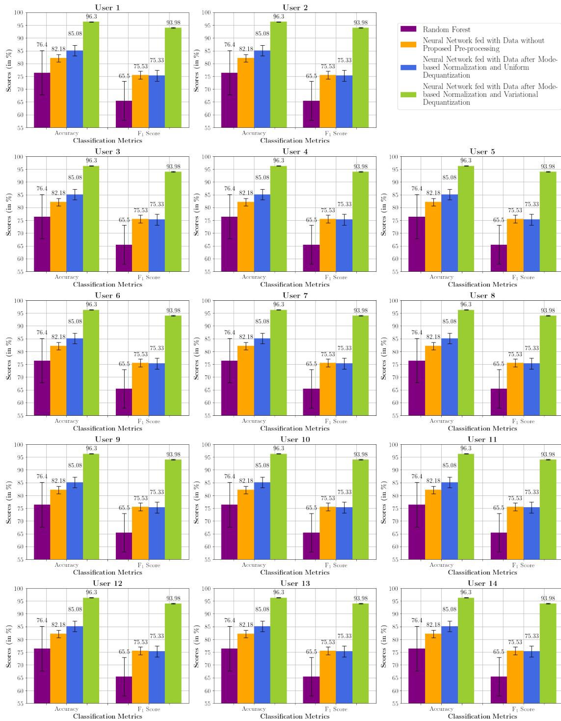
Figure 6.3: Personal thermal preference classification performance with standard deviation bounds for various ML models and data pre-processing methods.
