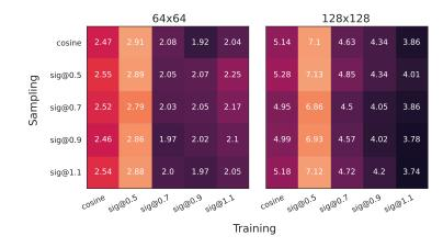
Figure 2.13: Effect of noise schedule. Comparing noise schedules for training and sampling, with corresponding FID score. The sigmoid schedule with an appropriate temperature is more stable during training than the widely used cosine schedule, particularly for larger images. For sampling, the noise schedule has less impact and the default cosine schedule can suffice.
