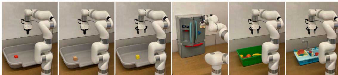
Figure 5.3: Real-world robotic tasks. We perform extensive real robot evaluations using a 7 DoF robot arm with a parallel jaw gripper. Our tasks include basic motor control skills (reaching a red block, pushing a wooden cube, and picking a yellow cube), variations in scenes (closing a fridge), objects (picking fruits), and scenes and objects (picking a detergent bottle from a cluttered sink).
