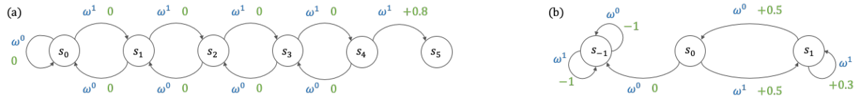
Figure 6.6: Multi-Step MDPs. (a) In the Chain environment, the society starts at state s_0 and the goal state is s_5 . Only activating primitive \omega_1 at state s_4 yields reward. The optimal global policy is to directly move right by continually activating \omega_1 . Without credit conservation, the society may get stuck going back and forth between s_0 and s_4 without reaching the goal. (b) In the Duality environment, the society starts at state s_0 . s_{-1} is an absorbing state with perpetual negative rewards. The optimal societal policy is to cycle between s_0 and s_1 to receive unbounded reward, but without redundant primitives, the society may end up in a suboptimal perpetual self-loop at s_1 .
