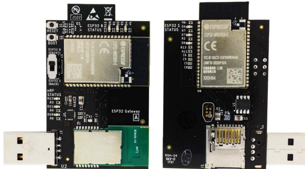
Figure 3.8: Gateway hardware. Our design distributes BLE, Wi-Fi, and 802.15.4 roles between two ESP32s and an nRF52840.
