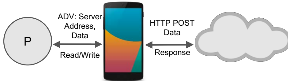
Figure 4.4: BLE Profile Proxy In default operation, the smartphone facilitates connection and profile-based communication between the BLE peripheral and the cloud endpoint specified in its advertisement.
