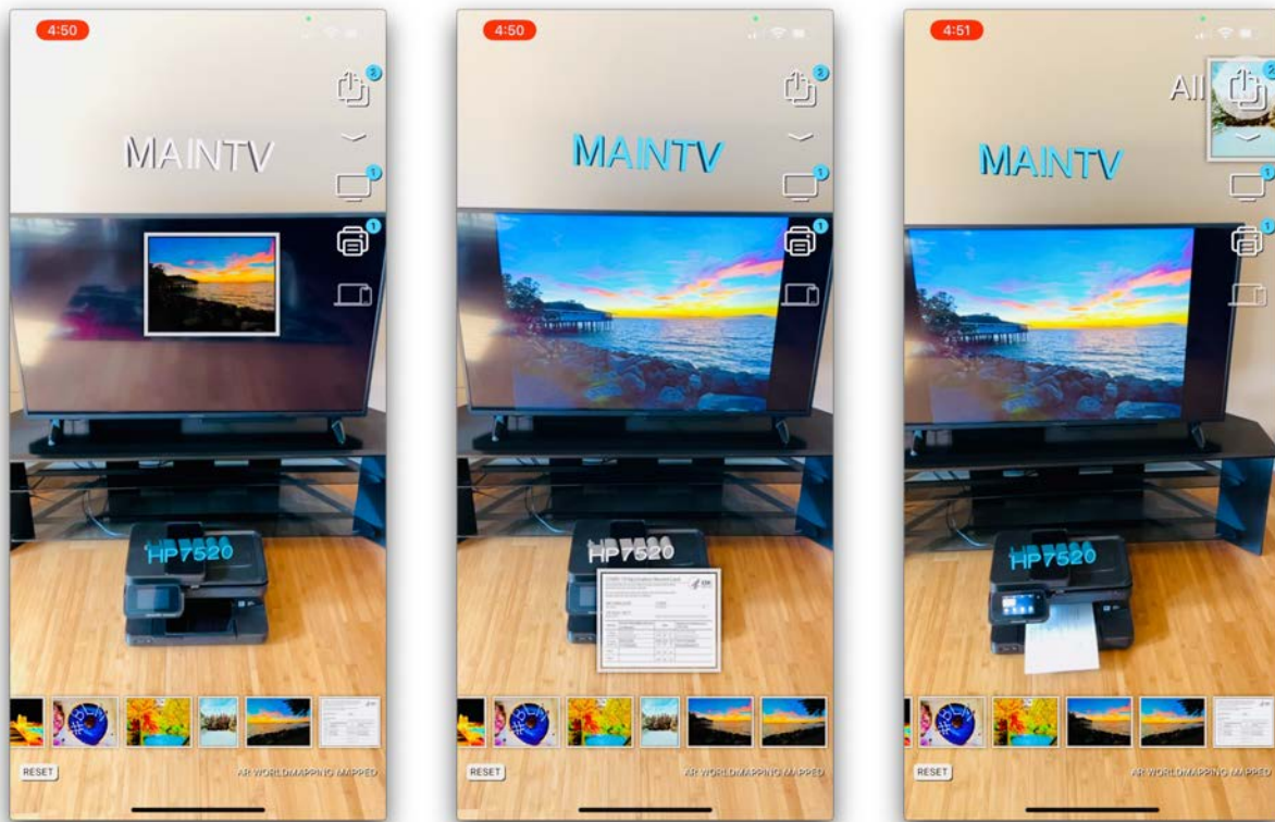
Figure 6.7: Application: Drag-and-Drop Share. A WebXR application that allows users to share images to network displays, printers, and computers, by dragging them to the device on the augmented camera feed. Users may also send media to all devices or all of a device type by dragging to corresponding on-screen action icons representing aggregates of all items in view.
