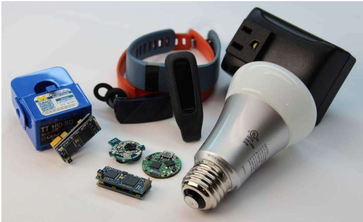
Figure 1.1: IoT Devices. Objects of a variety of form factors are embedded with an (often constrained) set of computational resources to create peripheral devices that enable “smart” capabilities in a variety of applications, such as lighting, power monitoring/control, personal health tracking, and environmental sensing.
