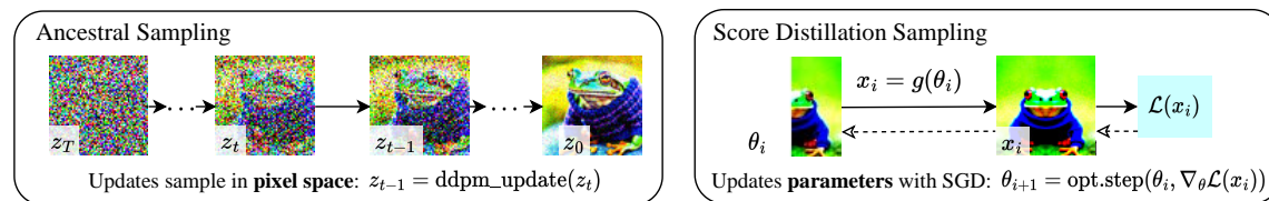
Figure 5.2: Comparison of 2D sampling methods from a text-to-image diffusion model with text “a photo of a tree frog wearing a sweater.” For score distillation sampling, as an example we use an image generator that restricts images to be symmetric by having \mathbf{x} = (\text{flip}(\theta), \theta) .
