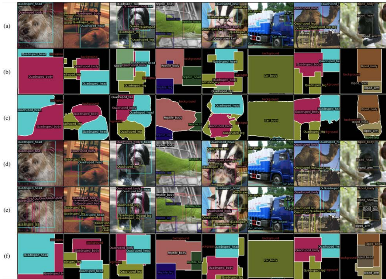
Figure 2.4: Deeplabv3+ and DINO Example Predictions (a) Original images with Ground Truth bounding boxes (b) Ground Truth segmentation masks (c) Deeplabv3+ Predicted segmentation masks (d) Deeplabv3+ Predicted segmentation masks converted to bounding boxes (e) DINO Predicted bounding boxes (top 10 only) (f) DINO Predicted bounding boxes converted to segmentation masks
