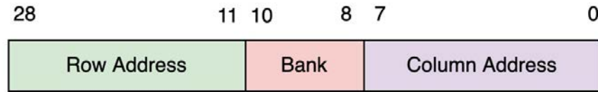
Figure 2.7: Breakdown of physical address.
