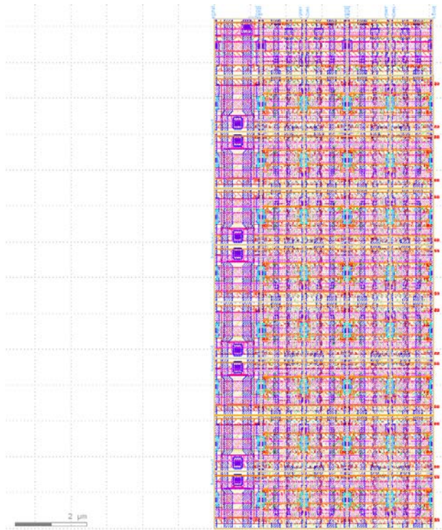
Figure 3.5: The center ninepatch cell for the bitcell array shown in 3.4.
