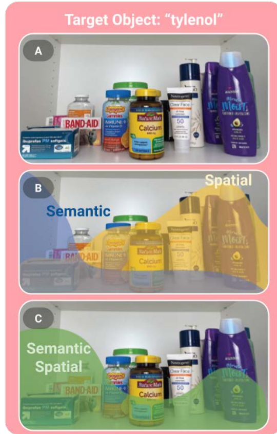
Figure 1.2: (A) Consider a robot search for a target object such as Tylenol in a semantically arranged environment such as a pharmacy shelf. (B) Semantic Spatial Search on Shelves ( S^4 ) computes a spatial distribution and a semantic distribution (see shaded areas) over where the target object could be. The spatial distribution is based on object shapes while the semantic distribution encodes likelihood of physical proximity (e.g., Tylenol is likely closest to Ibuprofen). (C) These are combined into a single semantic spatial distribution .
