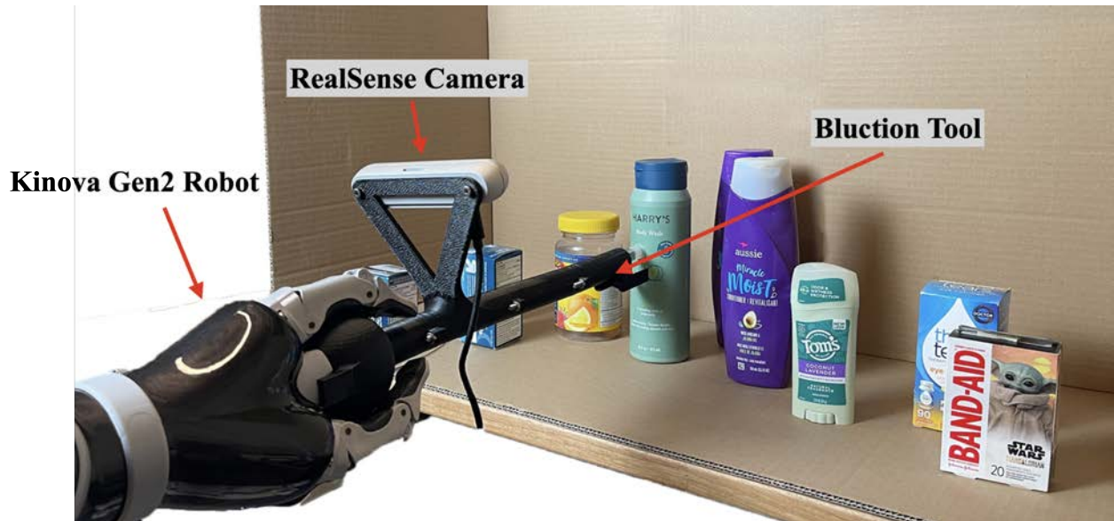
Figure 7.1: Physical setup with a cardboard shelf, pharmacy objects, Kinova Gen2 robot, a bluction tool [34] for extracting objects in the shelf, and an Intel RealSense RGBD camera mounted on the bluction tool.
