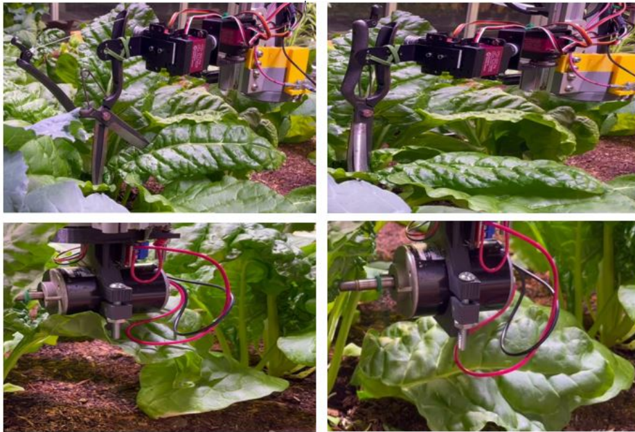
Figure 3.2: Pruning tools. Left: Physical model of Rotary Pruner with a high speed motor and trimming blades. Right: Physical model of Pruning Shears with three servos to control closing, tilt, and orientation.
