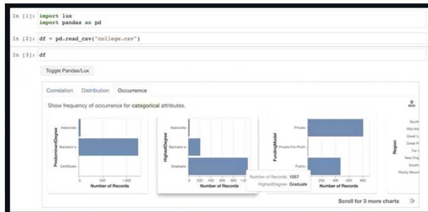
Figure 1.3: Example of Lux, a VisRec system, operating in a Jupyter Notebook Environment. The “college” dataset is rapidly ingested into a dataframe and then profiled and visualized with Lux in an eager fashion and in quick succession, with little to no user code.
