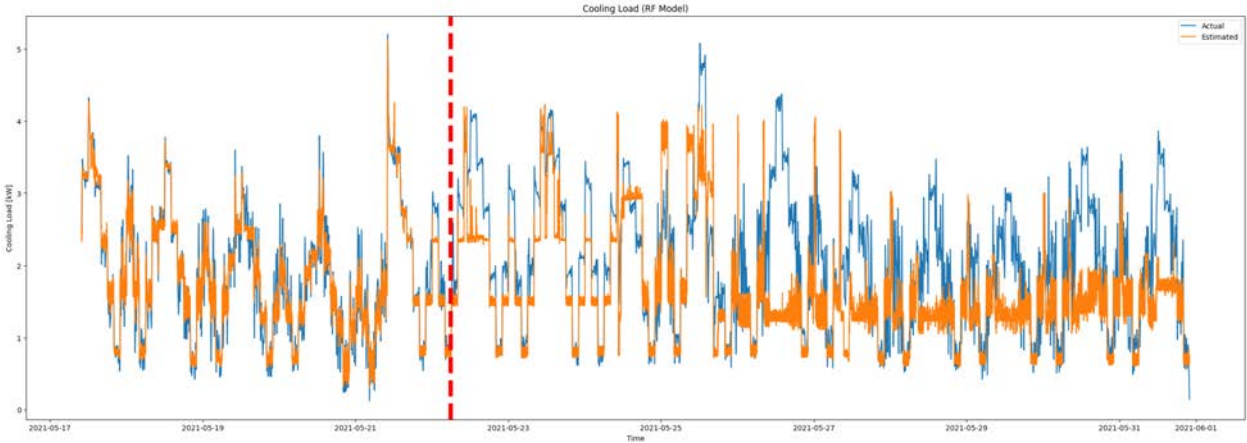
Figure 4.11: Comparison of measured and estimated cooling load data. The blue line represents the measured cooling load data, while the orange line represents the estimated cooling load data based on the RF model. The vertical red dotted line separates the training (left) and validation (right) data.
