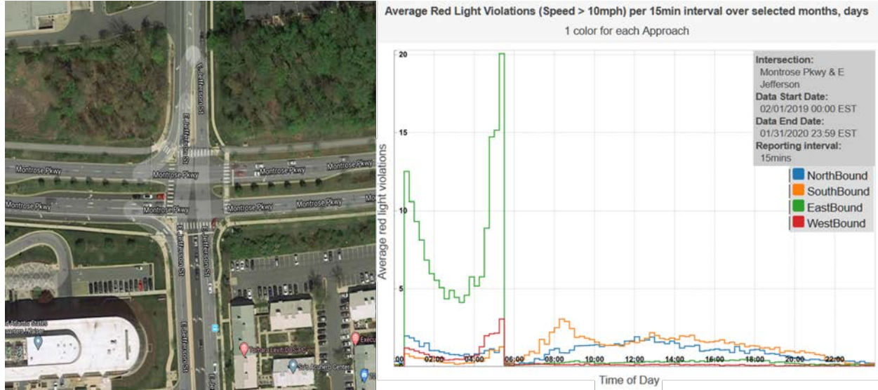
Figure 8.7: Intersection of Montrose Parkway and E. Jefferson Street in North Bethesda, MD: Statistics of red light violations collected over one year from 02/01/2019 through 01/31/2020.
