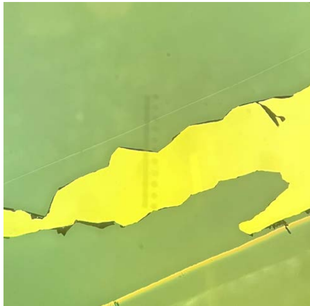
Figure 3.6: Au stack peeling after liftoff. The black strips are peeled back folds of the metal stack and the green is the glass wafer.
