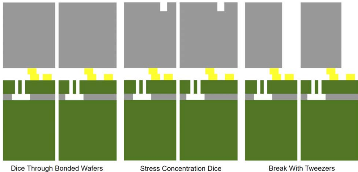
Figure 3.9: Process flow showing how to create 2 chips and expose pads through a full and partial dice where grey is glass wafer and SiO 2 , yellow is Au, and green is Si.
