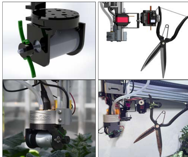
Figure 6.6: Pruning tools. Left: CAD and physical model of Rotary Pruner with a high speed motor and trimming blades. Right: CAD and physical model of Pruning Shears with three servos to control closing, tilt, and orientation.
