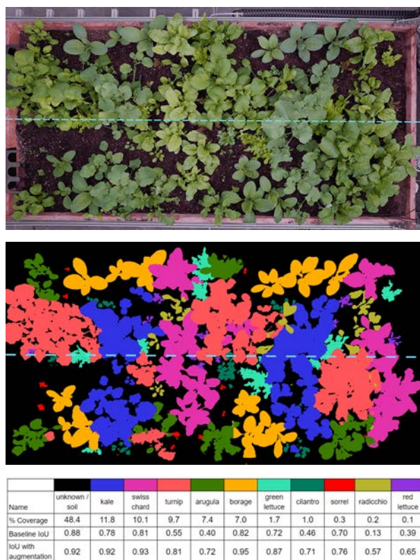
Figure 6.2: Learned Plant Segmentation Model. The figures above (from top to bottom) show an overhead image from October 6, 2020, and the classifier output from the network with augmented data. The overhead image is split in half as shown by the blue line. The top half is for training while the bottom half is for testing. Below, the table shows how much of the garden is covered by each plant and its respective IoU score based on the bottom half only. By adding augmented data, the model was able to more accurately classify unseen leaves when compared to the baseline with no augmented data. Low IoU for radicchio and red lettuce is consistent with a low percent of coverage.
