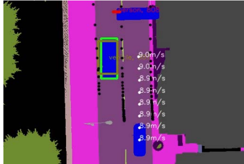
Figure 3.2: A bird’s eye view representation of an AV’s surroundings produced by the Pylot AV pipeline [27]. The representation is annotated with driveable regions, nearby vehicles, pedestrians, and the predicted paths of nearby agents.
