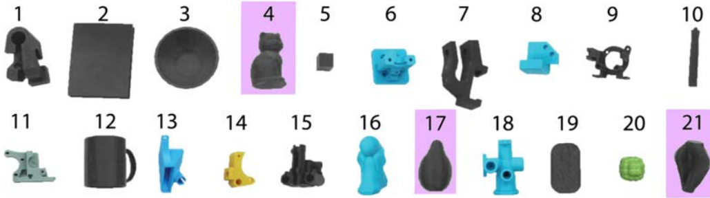
Figure 3.4: The 21 adversarial objects used in the grasp dataset collected by Danielczuk et al. [8], where analytic grasp models perform poorly. Each object is sampled with 25 test grasps, 5 trials per grasp. The training object set (cat, pear, vase) for our experiments is highlighted in purple.
