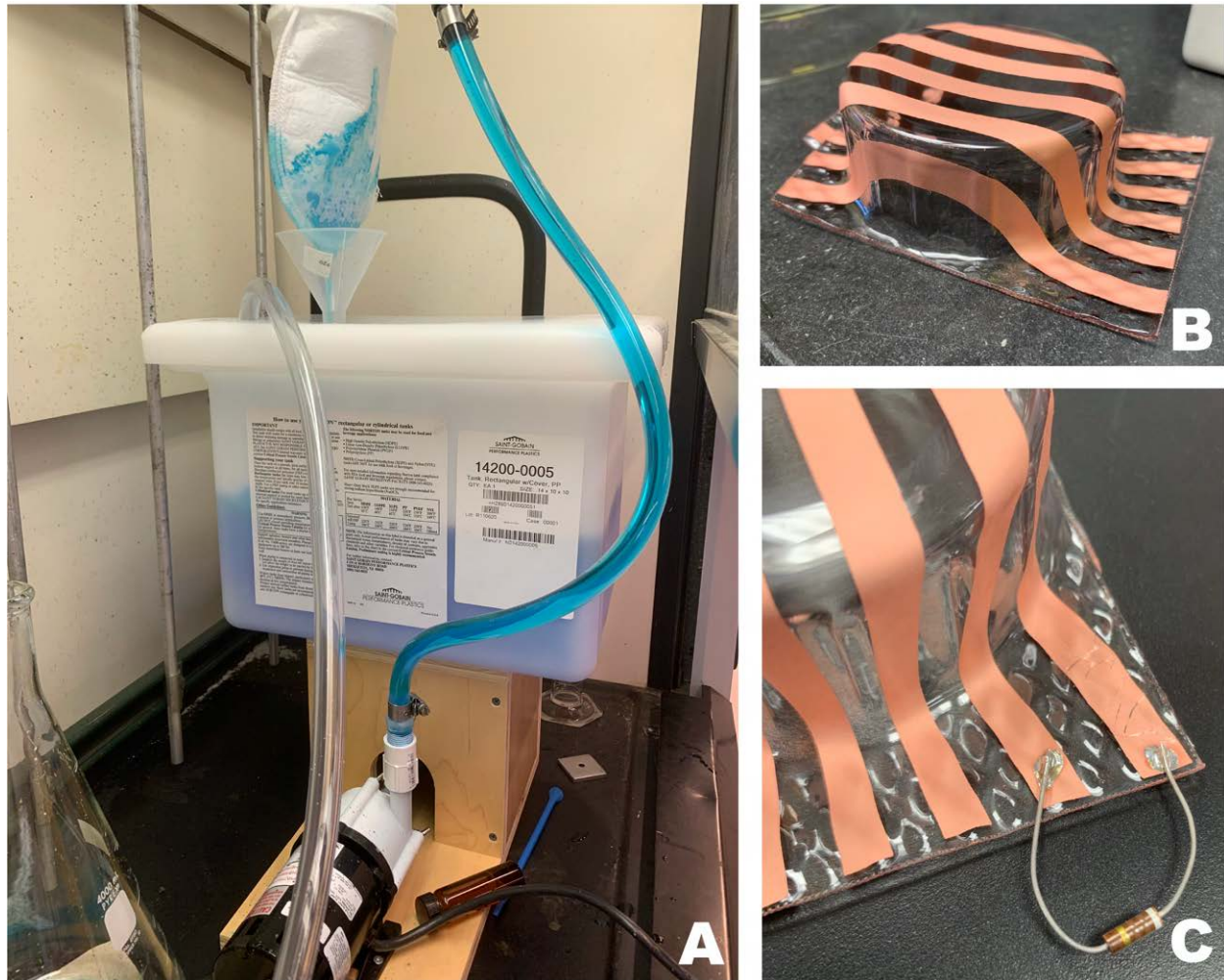
Figure 3.6: Electroless plating with a smaller sample. A) Our electroless copper plating setup including a polypropylene tank, circulation pump, filter bag, and nitrogen line. B) A small vacuum formed sample after copper plating to showcase the capabilities of our method. C) Demonstration of soldering a resistor to the plated copper traces.
