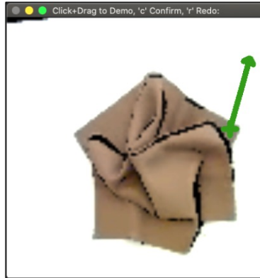
Figure 16.3: The user interface for human interventions. The current observation of the fabric state from the robot’s perspective is displayed, with an overlaid green arrow indicating the action the human has just specified.
