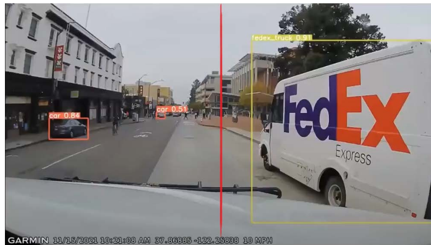
Figure 6.3: Vehicle detection and classification using YOLOv5 model. Bounding boxes include objects’ labels and confidence levels. Dashcam provides additional metadata: date, time, GPS coordinates, and speed of the bus. Red vertical line is the reference point for the illegal bus lane occupation analysis. FedEx truck is located in the right-hand side of the frame suggesting bus lane parking.
