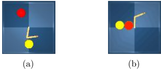
Figure 5.4: Reacher environment during demonstration time (a) and policy training time (b). During demonstrations, the uncertain region (red) is far from the robot arm (red) and the goal (yellow), but during policy optimization the goal position is randomized and sometimes the uncertain cost region is in the way forcing the agent to either go around or through it.
