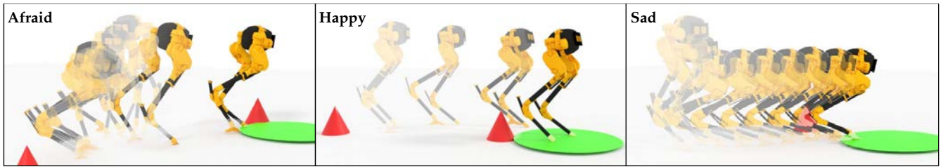
Fig. 4: Cassie must reach a target location avoiding obstacles represented by cones. Here it optimizes for various target emotions on various tasks using a model learned with our method. Visuals overlay one snapshot per second with earlier frames made more transparent. Afraid first takes a few cautious steps back before proceeding. Happy keeps head high and moves fast. Sad slouches and proceeds slowly.
