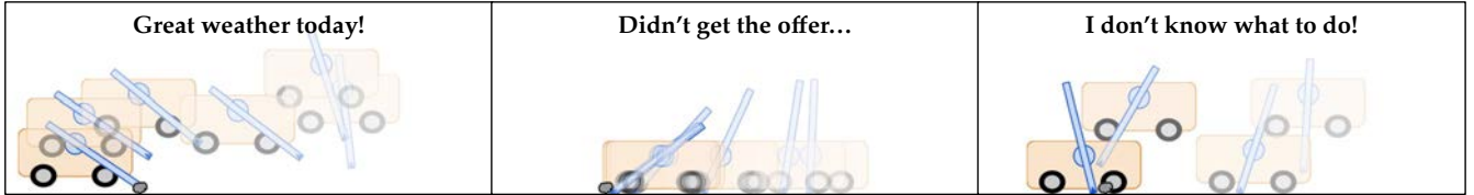
Fig. 8: Three trajectories for a single task where VacuumBot infers VAD from the displayed phrases and produces motions based on a study user’s trained model. When the human expresses cheerfulness it gracefully hops to the goal. When the human expresses sorrow it slowly slouches its way there. When the human expresses fear it reflects that nervous energy.
