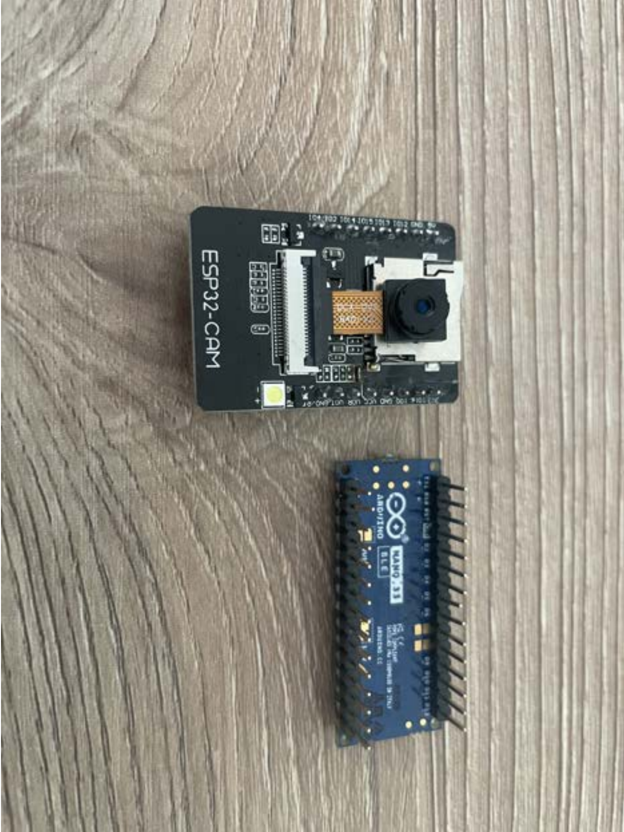
Figure 2.8: Left is ESP-32 Cam, Right is Arduino Nano BLE Sense
