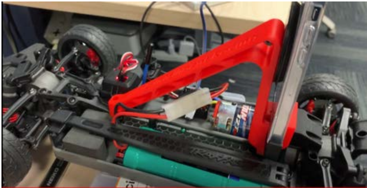
Figure 2.7: New iPhone mount with more structural integrity
