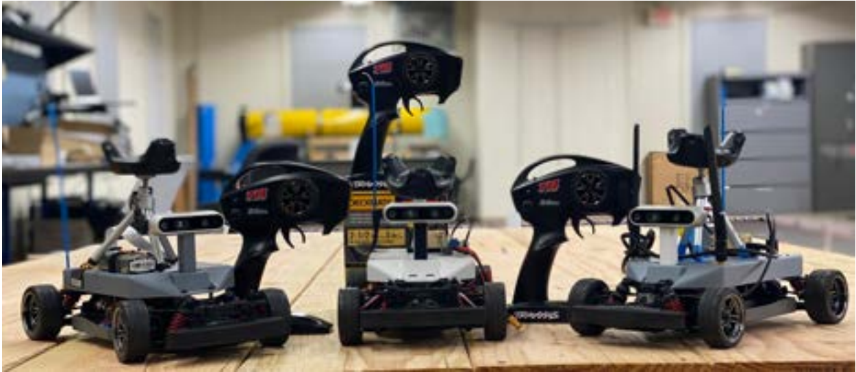
Figure 2.3: Original ROAR vehicle design with Vive Tracker
