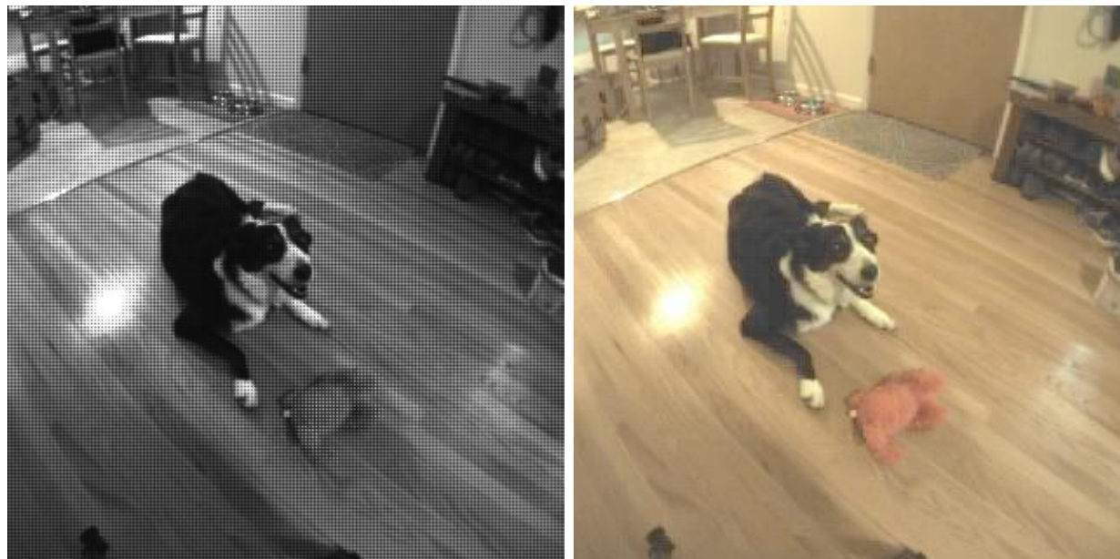
Figure 6.9: An image from Permacam, displayed as a mosaiced image (left) and demosaiced (right). Permacam is capable of capturing 320x320 resolution color images, which can be directly fed to machine learning inference tools for object, person, or in this case: dog detection.
