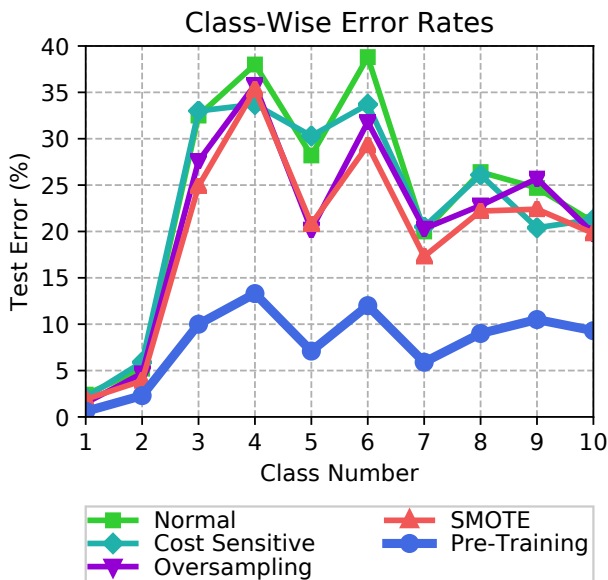
Figure 2.3: Class-wise test set error rates are lower across all classes with pre-training. Here the imbalanced dataset is a CIFAR-10 modification with imbalance ratio \gamma = 0.2 .
