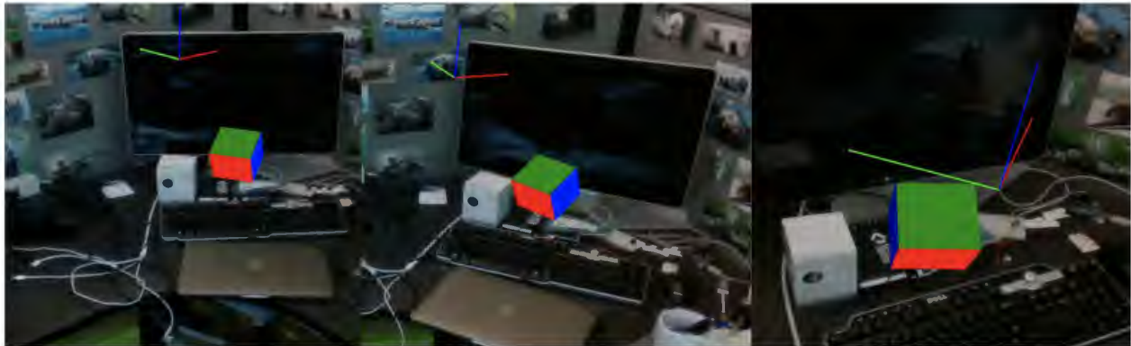
Figure 1.1: A visualization of the a virtual cube projected onto a camera image using the estimated camera position from OpenARK SLAM
