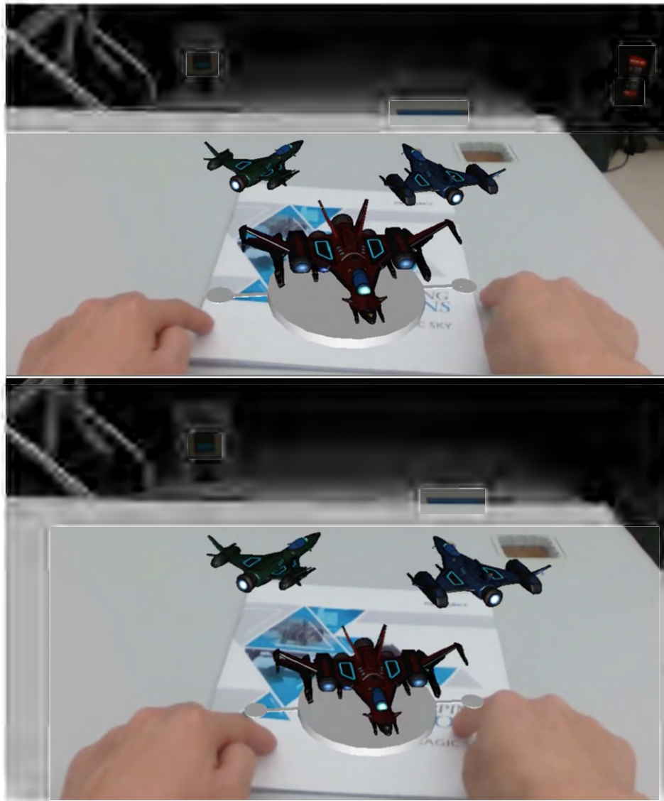
Figure 1.4: Example application built using OpenARK Hand Tracking. The user is able to scale the virtual object by touching the white dots and moving their fingers closer together or further apart
