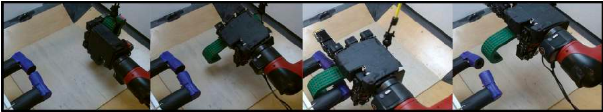
Figure 35: Filmstrip of the final learned rope hooking behavior. Using the user-provided milestones, our robot learns a set of skills that allows it to autonomously practice hooking and unhooking the rope (right two images) and recover from failure (e.g., after dropping the rope) by regrasping and reorienting the hook (left two images). After over 30 hours of unattended learning, our system successfully hooks the rope with over 95% success.
