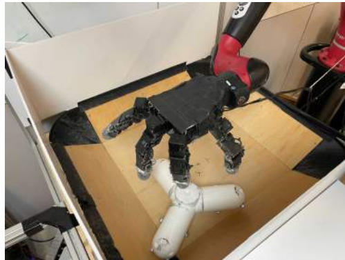
Figure 23: Real-world hand-arm manipulation platform. The system comprises a 16 DoF hand mounted on a 6 DoF Sawyer arm. The goal of the task is to perform in-hand reorientation, as illustrated in Fig 28 or pipe insertion as shown in Fig 29
