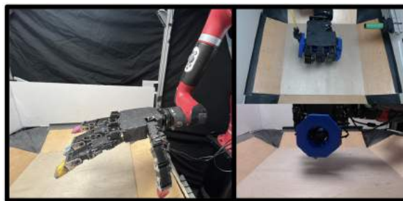
Figure 31: The robot consists of a 16 DoF hand mounted on a 7 DoF Sawyer arm (left). The workspace (right) is equipped with two RGB web cameras providing an overhead and side view.
