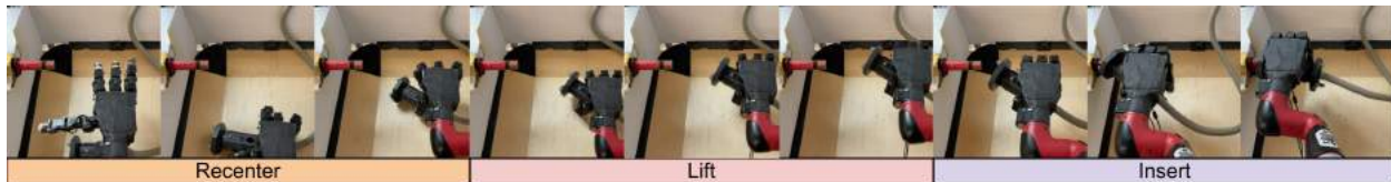
Figure 29: Film strip illustrating partial training trajectory of hardware system for pipe insertion. This shows various behaviors encountered during the training - repositioning the object, picking it up, and then inserting it into the wall attachment. As seen here, MTRF is able to successfully learn how to do pipe insertion without any human intervention.
