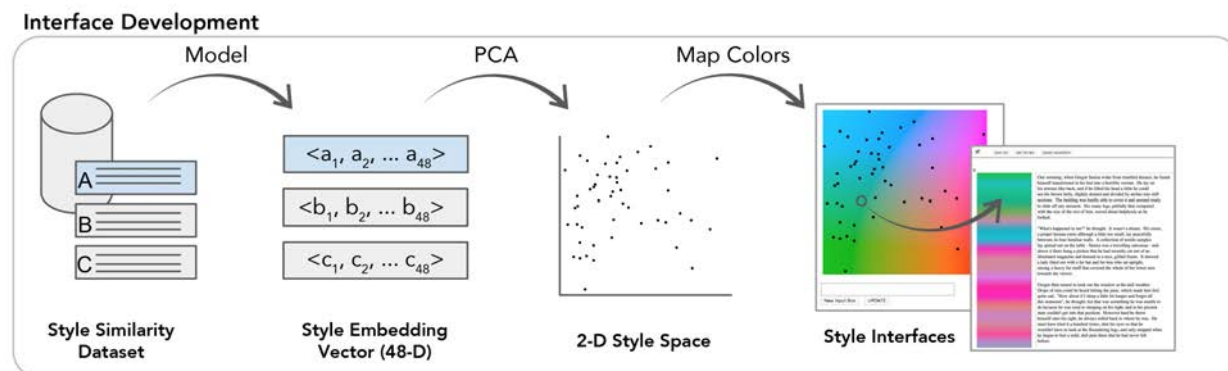
Figure 3.4: Interface design method. From left: Style comparisons from the collected dataset are used to train a predictive model, which learns a high-dimensional vector embedding associated with how people perceive style. The embedding is projected to 2 dimensions using principal component analysis (PCA). By mapping a color space to the 2D projection, the style of text excerpts can be associated with a color, and used to create interactive experiences (Left Interface: Explorer; Right Interface: Editor).
