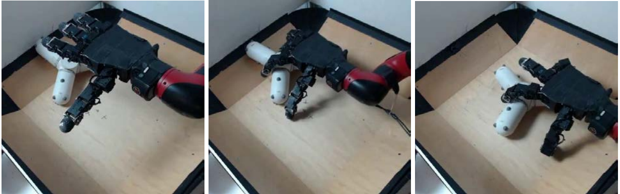
Figure 27: Utilizing prior data for online learning allows us to solve challenging real-world robotics tasks, such as this dexterous manipulation task where the learned policy must control a 4-fingered hand to reposition an object.
