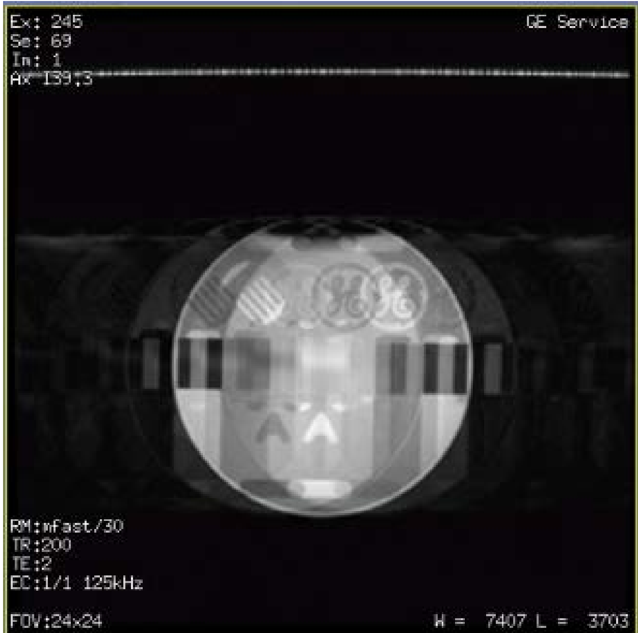
Figure 11: Example reconstruction of a FIESTA image acquired with an extremely large TR (200 ms) showing severe motion artifacts. In this case, the exaggerated TR is used to show the "worst case scenario" for slow pulse sequences and highlight the artifact BPT can be useful in correcting.
