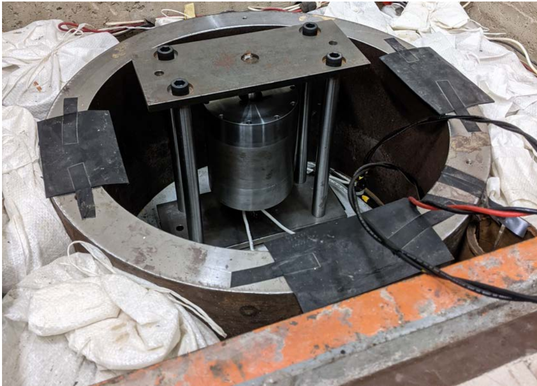
Figure 6.5: Machine assembly containment. The sandbags, steel cylinder, and machine assembly can be seen in the picture.
