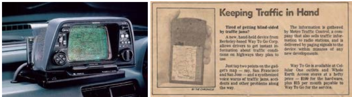
Figure 2.7: Left: Onboard navigation unit prototype built by Honda in 1981 for route guidance. Right: Newspaper commercial for Way to Go aftermarket device circa 1990, one of the early prototypes of navigational apps built by UC Berkeley.
