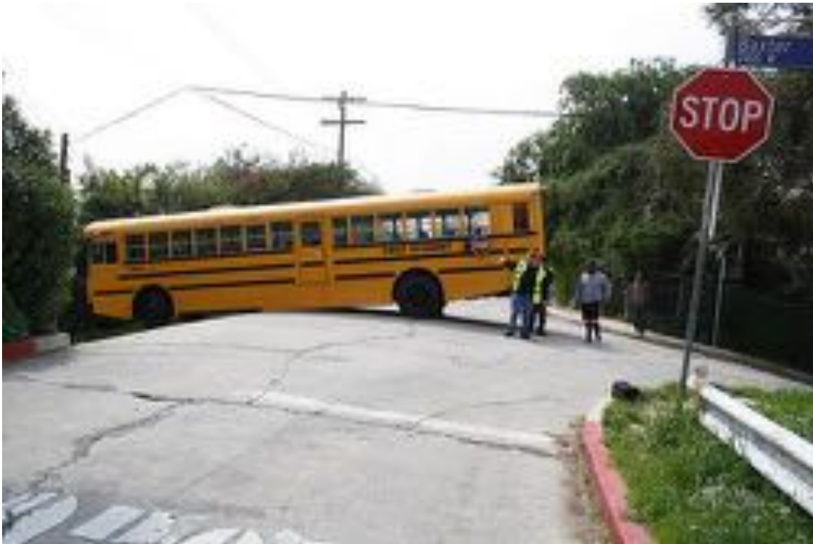
Figure 4.9: Bus crash because it was routed on a road too steep. Photos by Ingrid Peterson via Flickr.
