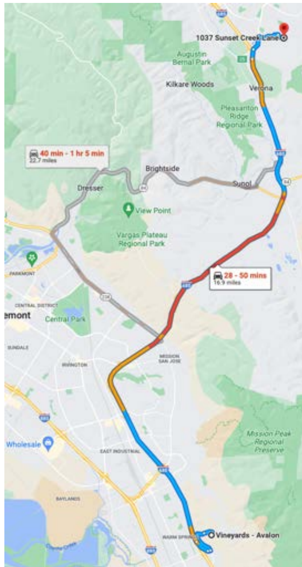
Figure 2.8: July 14 th , 2022 4:30 pm, traffic guidance on Google Maps within the Fremont, CA area. The request is done on July 13 th and uses the Google Maps traffic prediction system. The first route suggested (in blue, orange, and red) uses a local road, then a collector road, then a minor arterial road, and then an interstate before using a minor arterial, a collector, and then a local road to reach its destination. The road categories of the road used by the trip increase and then decrease. However, in the second road suggested (in grey), this is not the case: a major arterial, a minor arterial, and a collector road are used between the same interstate road.
