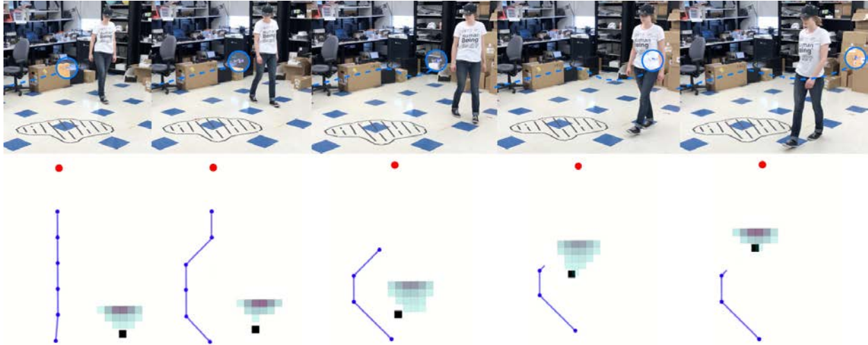
Figure 3.9: Inferring \beta leads to predicted state distributions whose entropy increases whenever the utility model Q_H fails to explain observed human motion. The resulting predictions are more robust to modeling errors, resulting in safer motion plans. Here, the quadcopter successfully avoids the pedestrian even when she turns unexpectedly.
