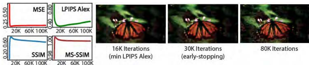
Figure A.2: Early stopping for 2D experimental images. The reconstruction gets noisier after converging to the lowest LPIPS score. In the main paper, we show results with early stopping for our experimental data; interestingly we don't see this effect on simulation data perhaps due to the lack of noise and model mismatch.
