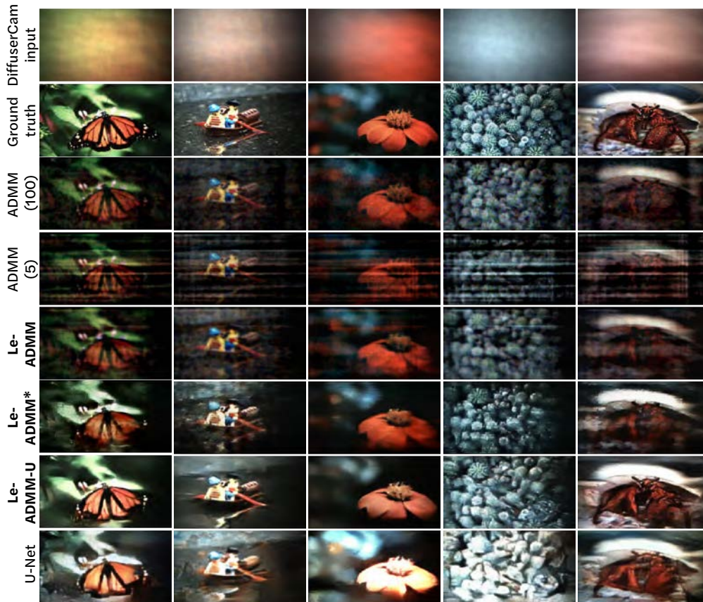
Figure 4.4: Test set results , with the raw DiffuserCam measurement (contrast stretched) and the ground truth images from the lensed camera for reference. Le-ADMM (71 ms) has similar image quality to converged ADMM (1.5 s) and better image quality than bounded ADMM (71 ms). Le-ADMM* and Le-ADMM-U have noticeably better visual image quality. The U-Net by itself is unable to reconstruct the appropriate colors and lacks detail.
