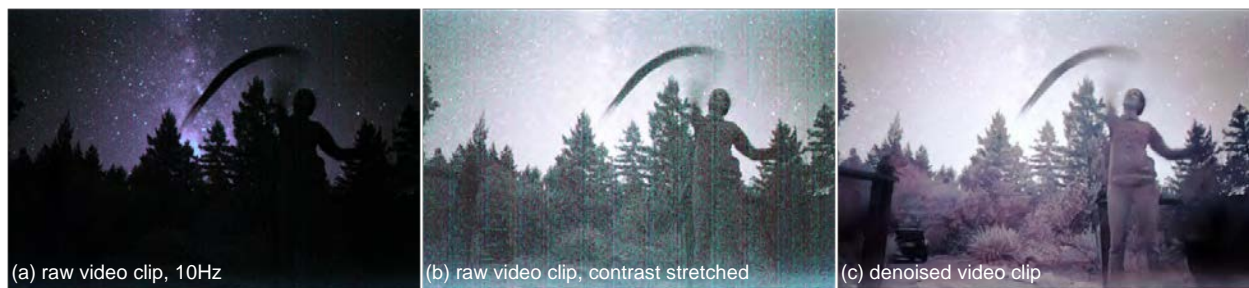
Figure 7.1: Video denoising in submillilux. (a) Raw noisy video clip (10fps video) taken between 0.6–0.7 mlx (millilux) on a clear, moonless night with no external illumination. (b) Result after contrast stretching the video clip. (c) Denoised video using our denoiser.
