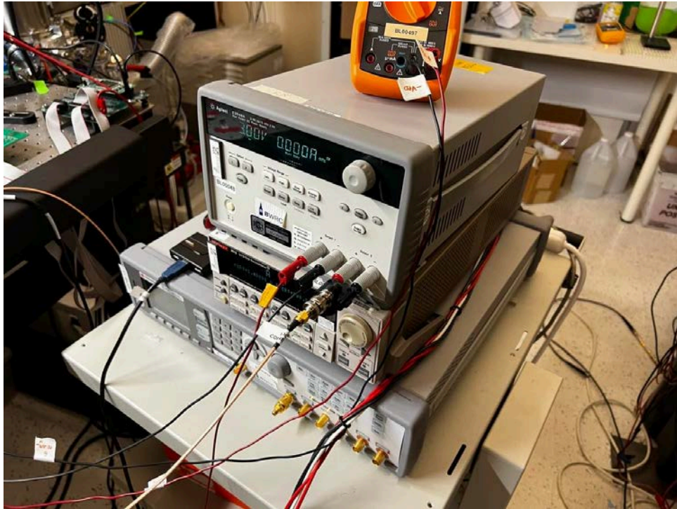
Figure 19: Sourcemeter, Power Supply, and Multimeter for TIA testing
