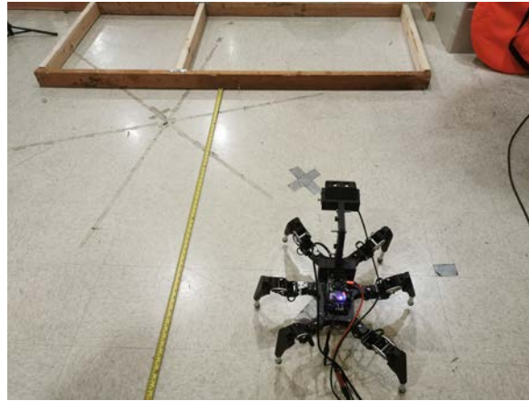
Figure 2.18: Test 1: hexapod starts at 1m from 10cm joist. The resulting grid map images and line detections for this experiment are shown in Appendix A. Demo video .
