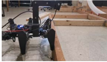
(a) Pose 1: stop near joist, calculate trajectory
