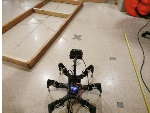
Figure 2.23: Test 6: hexapod starts at 1m from 75° oriented joist. The resulting grid map images and line detections for this experiment are shown in Appendix F. Demo video .
