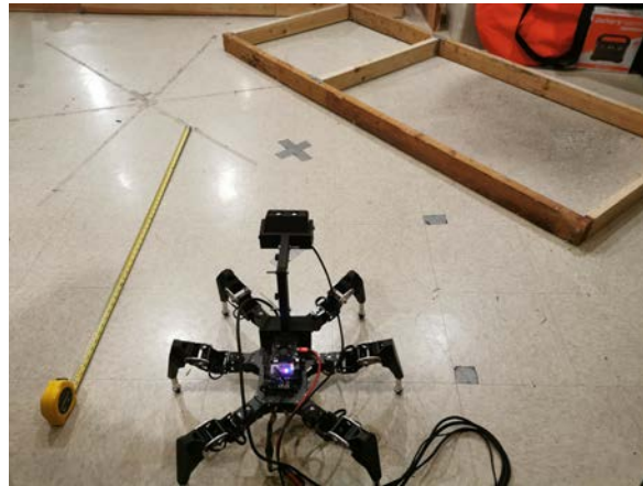
Figure 2.21: Test 4: hexapod starts at 1m from 45° oriented joist. The resulting grid map images and line detections for this experiment are shown in Appendix D. Demo video .
