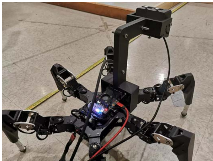
Figure 2.13: Experiment to evaluate the vertical and horizontal FOV of image with different pitch angle configurations
