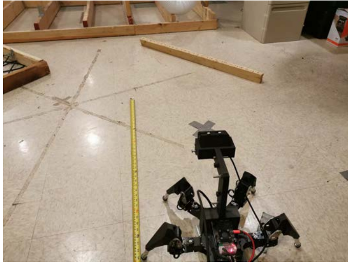
Figure 2.16: Joist are oriented at 1m in front of the hexapod.
