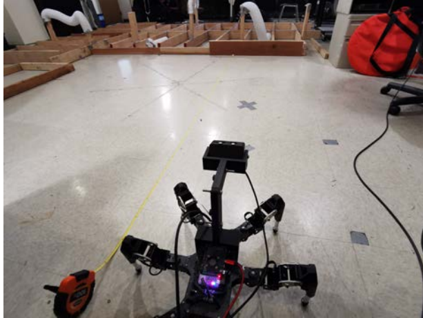
Figure 2.24: Test 7: hexapod starts at 2.7m from 18cm joist. The resulting grid map images and line detections for this experiment are shown in Appendix G. Demo video .
