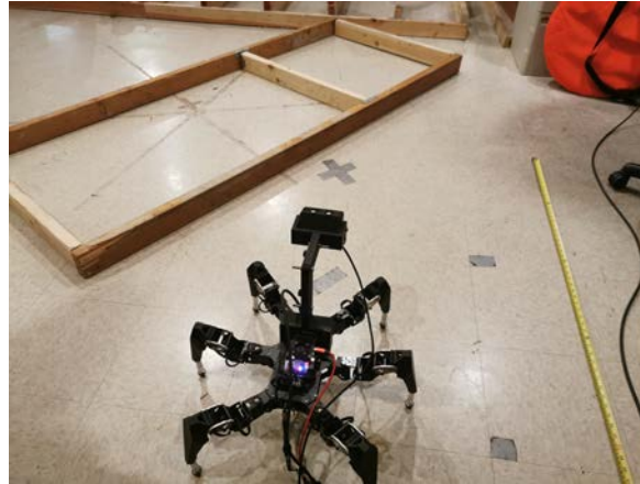
Figure 2.22: Test 5: hexapod starts at 1m from 60° oriented joist. The resulting grid map images and line detections for this experiment are shown in Appendix E. Demo video .
