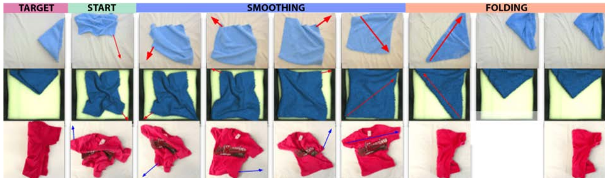
Figure 3.6: Full Folding Sequence: The first and second row is a time-lapse of a sequence of 6 actions taken by the YuMi and dVRK respectively, and with actions overlaid by red arrows, to successively smooth a wrinkled fabric and then fold it according to task 3 in Section 3.6. The third row is a time-lapse of a sequence of 5 actions taken by the YuMi to complete task 10 in Section 3.6. Here, robot actions are overlaid with blue arrows.
