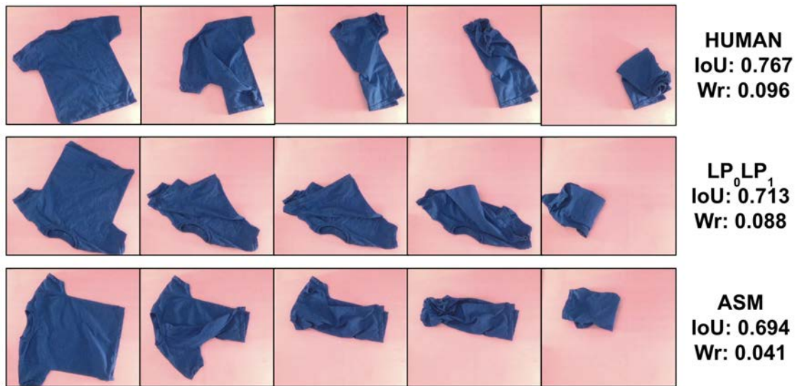
Figure 5.7: Representative episodes of the folding subtask executed by HUMAN (Row 1), LP 0 LP 1 (Row 2), and ASM (Row 3). LP 0 LP 1 and ASM achieve performance competitive with human teleoperation.
