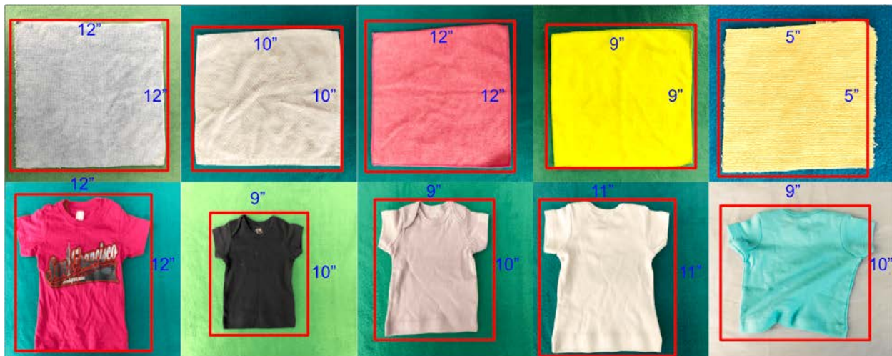
Figure 3.4: Fabric Specifications: Images and dimensions of the square fabrics and shirts we use in experiments.
