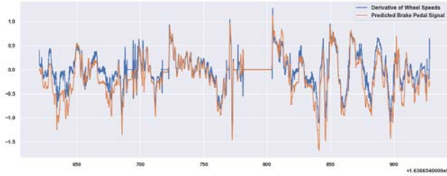
Figure 4. Predicted Brake Pedal Signal and Acceleration. The smoothed derivative of the wheel speeds was compared to the predicted brake pedal signal, showing a strong relationship between the two signals. The Pearson correlation coefficient between these two timeseries is 0.92.
