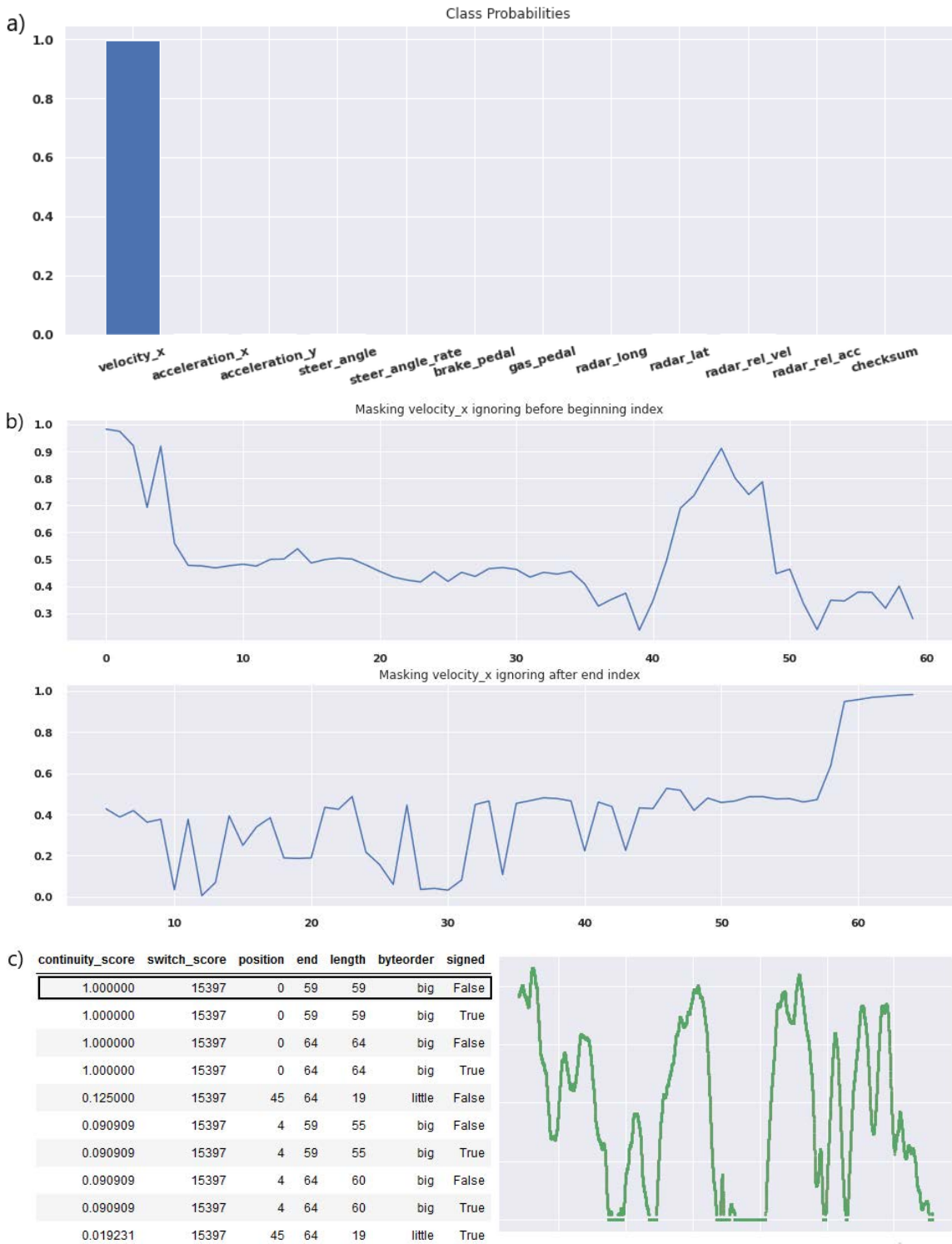
Figure 3. Bit boundary masking for likely wheel speed signal on test Nissan data. a) The model predicts the CAN message to only contain a velocity signal. b) The masking process generates peak values at possible beginning and ending bit positions. c) Through the scoring process, an encoding is chosen. The encoding is applied to view the raw velocity signal.
