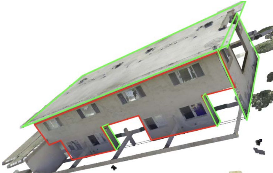
Figure 3.2.: Example of proximity detection for the base facade which is shown in red; the neighboring facades are shown in green. Some of the neighbors correspond to actual facades of the building and some are "junk" e.g. fences
