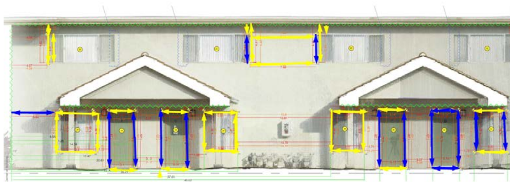
Figure 4.17.: Example of larger than 0.06 feet vertical errors in West-Elevation of Corona 205 shown in blue, less than 0.06 shown in yellow; total of 28 vertical measurements and 37 horizontal measurements
