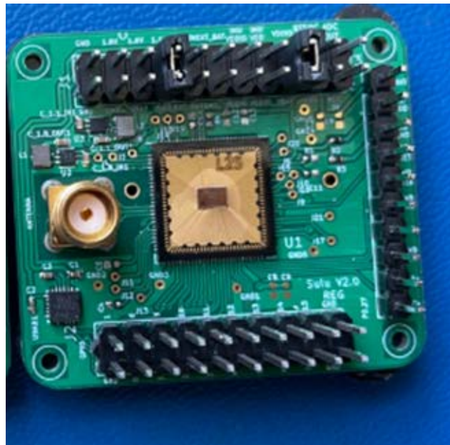
Figure 2.3: Fully assembled Sulu v2 development board. GPIO (bottom 2 rows of pin headers), power connections (top 2 rows of pin headers), and external communication connections (right row of pin headers)
