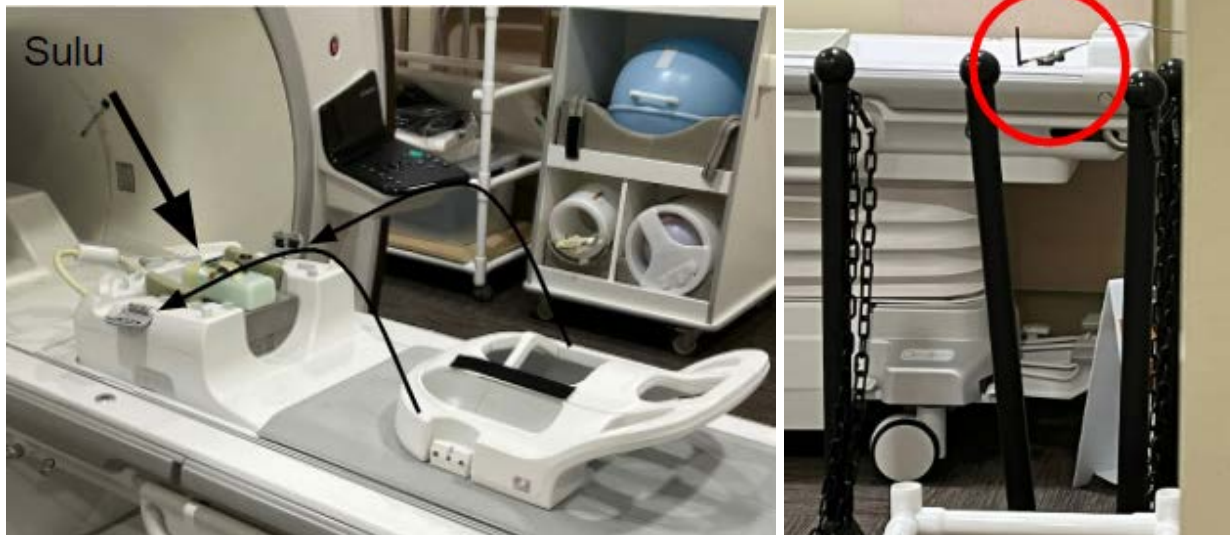
Figure 3.8: Close-up of semi-open structure SC \mu M Sulu development board was placed within with MRI coils designed by Julian Maravilla intended to be used in combined TMS-EEG-fMRI project. The total overall structure was tested both in the bore as pictured in figure 3.7 and on the bed of the scanner pictured here (left). Openmote B with antenna and high pass filter in the corner of the scanner room connected through the conduit into operator room (right).
